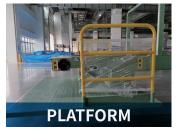
Increase loading and unloading convenience. personnel can stand on the telescopic conveyor head position for loading and unloading of goods, reduce manual handling intensity.
