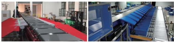
An intelligent cross-belt sorter with a high degree of space utilization. Suitable for narrow and long processing site.
